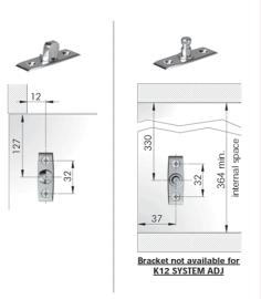
The dimensions of the above drilling plans refer to carcases which use standard sprung or unsprung hinges and mounting plates 0 mm. Please note that the opening angle varies with respect to the hinge brand and adjustment carried out.
