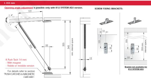
The dimensions of the above drilling plan refer to carcases which use standard unsprung hinges and mounting plates 0 mm. Please note that the opening angle varies with respect to the hinge brand and adjustment carried out.
